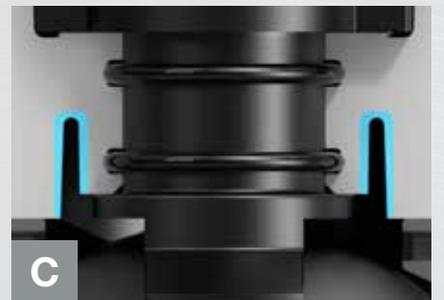
**C** The **flexible spindle shaft** ensures equal compression around the O-rings when loaded by internal pressure. At the same time the groove will adapt to any deformation as a result of upstream pressure on the ball when the valve is in the closed position.
