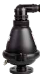
Series 701/75 Combination air valve Orifice sizes: Automatic: 12 mm 2 Kinetic: 804 mm 2 Reinforced nylon Inlet flange or 2 1/3" BSP thread PN 10 DN50-100
