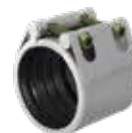
Series 745/20 Repico® slip coupling Universal for all pipe types Non-tensile Stainless steel AISI 316 NBR or EPDM sealing DN15-600
