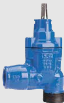
Series 11/30 - angle valve with external thread on inlet and tensile resistant socket joint for PE pipes on outlet.
