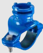
Series 100/14 - Tapping saddle for iron/steel pipe, Ø60-223 mm, ductile iron.
