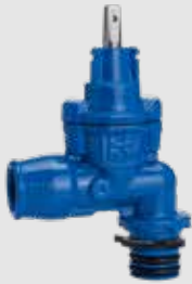
Series 103/31 - Service connection angle valve with one Supa Lock™ spigot end and one Supa Lock™ push-in socket end for PE pipes Ø32-40 mm, ductile iron.
