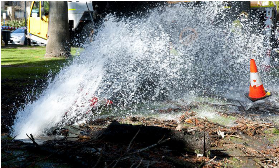
Severe water pipe burst caused by damaged pipework
